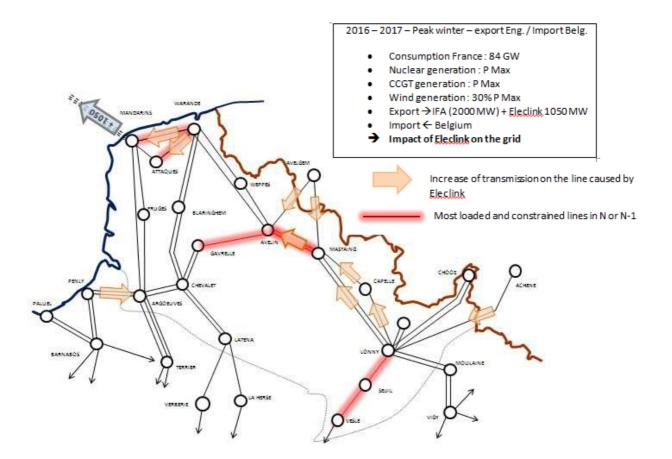
The exports following the insertion of Eleclink f(1,050 MW) increases flows on the Avelin-Mastaing 400-kV lines. If one the two transmission lines is lost, the second could therefore be constrained...
