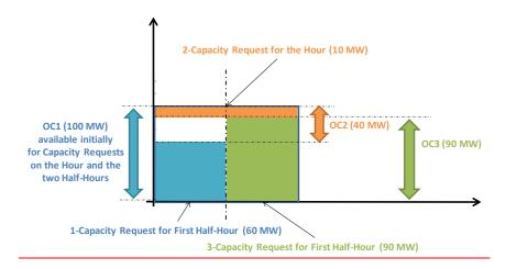
The first capacity published for allocation for the Hour and the two Half-Hours is OC1 (100 MW). Given the amount shown in the above figure, the following applies:
