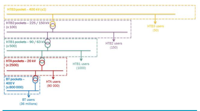
Figure 2 : Breakdown of the grid into pockets (order of magnitude)
