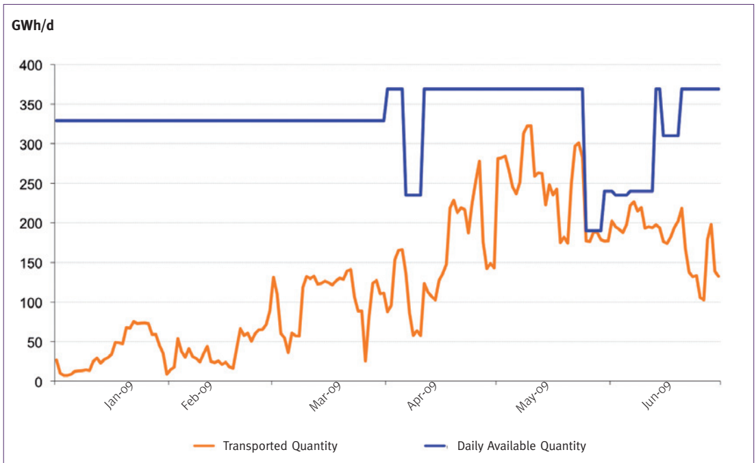
FIGURE 17 – Use of capacity at the Midi Network Interconnection Point from GRTgaz South to TIGF - in GWh/day, January - June 2009 -
